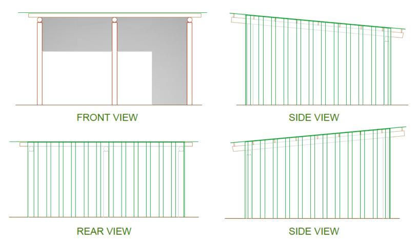
RUSTIC TIMBER FRAMEWORK (TELEGRAPH POLE UPRIGHTS AND CROSS MEMBERS. SCAFFOLDING PLANK ROOF TRUSSES. THE REAR,TWO SIDE ELEVATIONS AND ROOF CLAD WITH METAL PROFILE SHEETING (DARK GREEN). FRONT ELEVATION LEFT OPEN FOR EASE OF VEHICLE MANOEUVRE.
